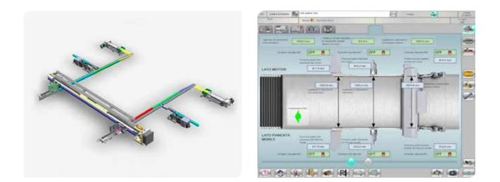
Thanks to the new motorized adjustment system, regulating the angle of the guides at the PCR infeed is now much simpler. The PCR interface has a dedicated page illustrating the positions of the actuators and their operation. This system ensures perfect powder loading and slab edge density at all times.
